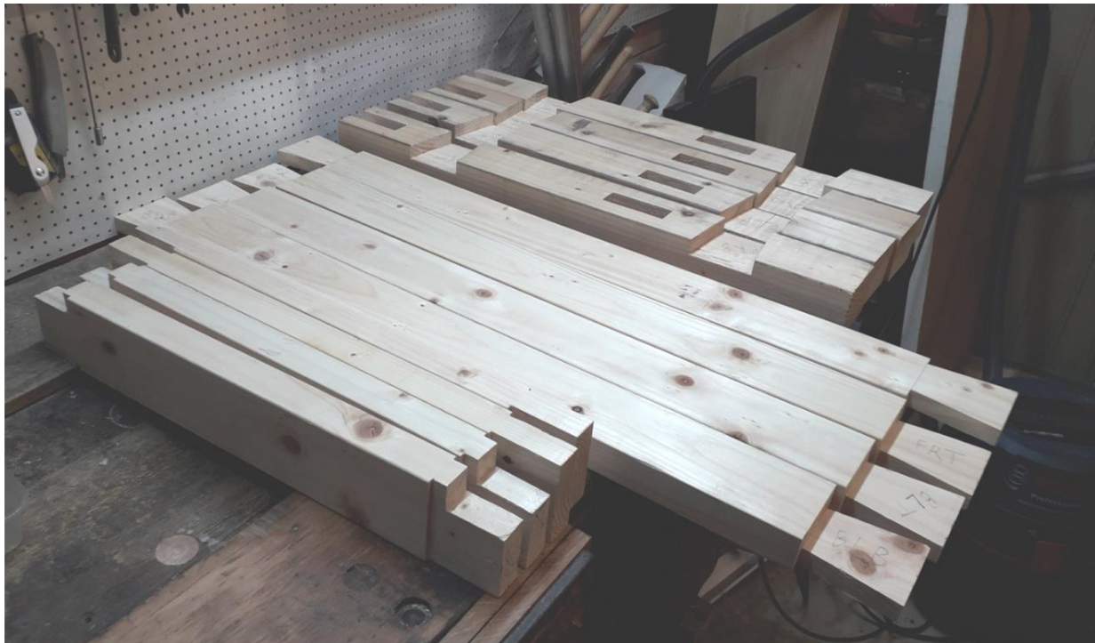
All the joints cut (8 mortice and tenons, 4 with haunches, and 8 lapped dovetails)
