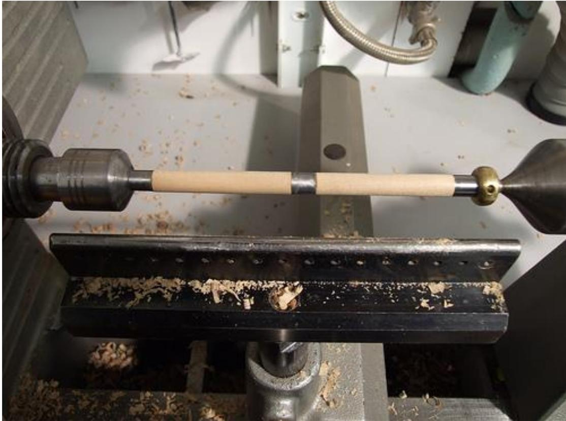
You need to sand the barrels to a fine finish. I generally start with 240 or 320 grit and work down to anything up to 1200 depending upon the quality of the kit I am making. I use j-flex or Abranet.
