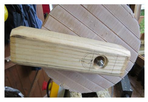
Now for the bit of off centre turning for the transition from shaft into the handle.
