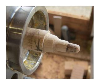
The next thing to work out was how to hold the pieces whilst turning. I used 12mm beech dowel held in the centre of my chuck, then turned the dowel to a tight fit stepped for both the 6mm and 10mm holes then tightened up with the live centre.
