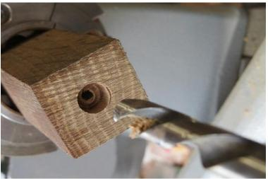
I started by drilling 6mm through the centre of each piece on the lathe, then a 10mm hole about 5mm deep at each end. I only did that on the first one, because I realised that as I was holding a not so square piece of timber in my 50mm jaws and that the 10mm x 5mm hole was not guaranteed to be central. Μv intention was for that 10 x 5 hole at each end to hold glue for added strength.
