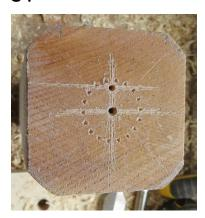
Offset centre for turning the hand holding part of the True centre for turning to remove corners.
