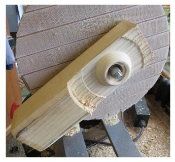
Then back to between centres, but this time offset to retain the transition section at the bottom of the handle. Then turning the hand holding part of the handle.
