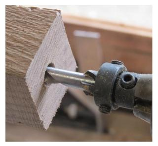
My solution to this was to use a combination 6mm drill bit/counter bore bit (part of a set I won in the club raffle) This would still give me that hole for extra glue. I centred using the 6mm drill bit part, prior to tightening the jaws.
