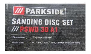
I purchased again from Lidl a box of 30 number 225mm diameter loop backed sanding discs 6 of each grade 60/80/120/180/240. I used them on the lathe with a Faceplate Ring fixed to an MDF disc plus hook backing on the face. I think they cost around £3 to £4 that is a fraction of what you would pay elsewhere. They where originally being sold for use with a dry ling system sander but are ideal for our usage.
