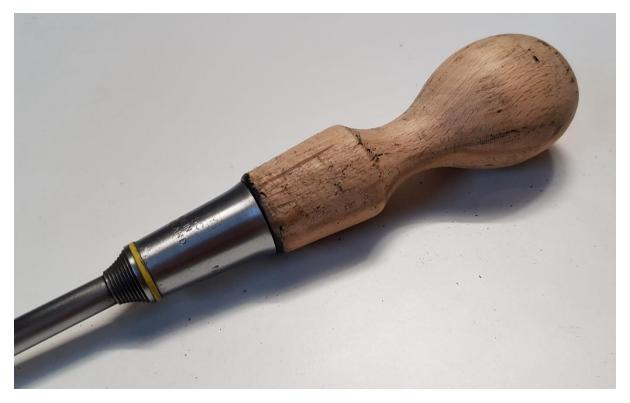
Careful sanding by hand finishes the job and prepares the handle for a new coat of paint. Almost good enough for an oil or lacquer finish but not quite.
