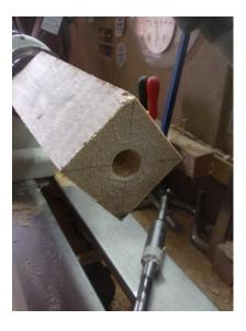
Locate the timber in the chuck and using a 25 mm Forstner bit in a Jacobs chuck and drill out to a depth of 170mm, this is to take a 150 mm. Because the 25 mm Forstner bit was not long enough I fitted it in to an extension. The depth is to give a bit clearance at the bottom of a test tube and an 8mm hollow at the top of the vase and also for the lip of the test tube to sit in just right and therefore not resting on the bottom of the hole.
