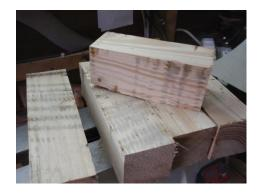
Cut into the desired length removing the parts with shakes in them but remembering to allow for a good chucking point and room for parting off.
