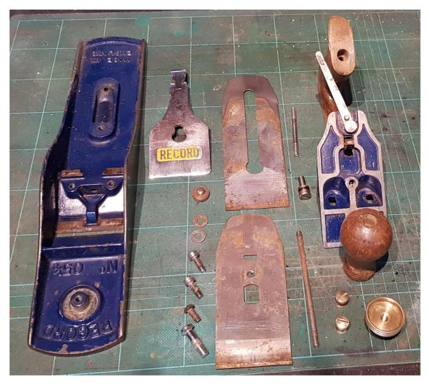
I reshaped the handle to remove the damage, sanded and stained both knob and handle with an Indian rosewood stain and sprayed them with acrylic lacquer. All metal parts were de-rusted with a brass wire wheel or 3M abrasive wheel as necessary, the blade sharpened, and all components oiled and reassembled.
