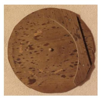
I could now mount the timber onto the dowel through any of the 13 holes. So, by using the 6 holes marked "A" I could turn the rings to 10mm deep on one side, then turning the piece over I turned the other rings using the holes marked "B" to 10mm deep. Each time I put three wood screws with a washer at the head through three of the unused 6mm holes, to hold the piece to the face plate.
