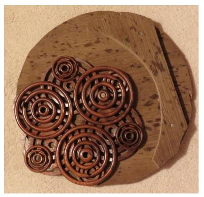
This photograph gives you an idea of how I used each centre. Basically, it was turned using only parting tools, there was however a lot of cleaning up with files and abrasive off the lathe.
