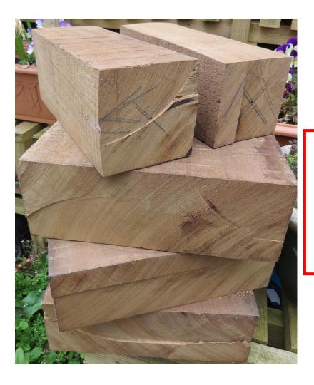
My hand-held circular saw only cuts to a depth of around 50mm so I had to cut from both sides.
