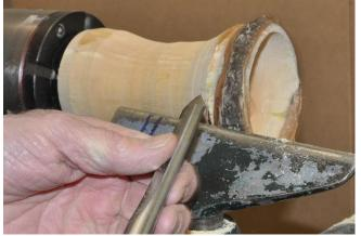
I have been taking very light cuts at the free edge with a sharp tool but a large area of bark has separated and has been lost.
