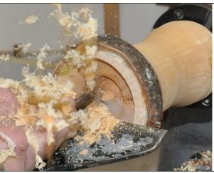
The final smooth shape to the inside of the bowl can be formed with a scraper. I am using a 1" negative rake round nosed scraper.
