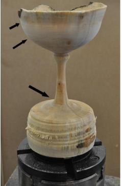
Now that those problems have been sorted, we can part off the goblet starting with a parting tool with the lathe spinning and finishing with the lathe stopped using a fine saw.
