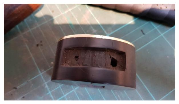
I polished up the brass repair plate and faceplate, drilled and tapped the repair plate for a new locking screw and reassembled the body.
