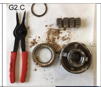
. Each carrier is stamped with a numbers 1-4 (see picture G2.E). For the Nova G2 chuck there is no need to record which slot the individual carrier came from.
