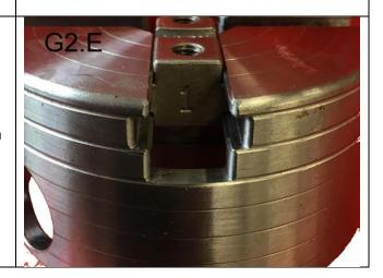
Now insert all the other carriers in order 2-4 into slots in a **clockwise** sequence. Bring the carriers together so that their inner edges form a square and turn the whole over (G2. F). You can now drop the lubricated scroll onto the jaws and with a little 'jiggling' it will engage with the carriers. Now replace the circlip and the job is complete.
