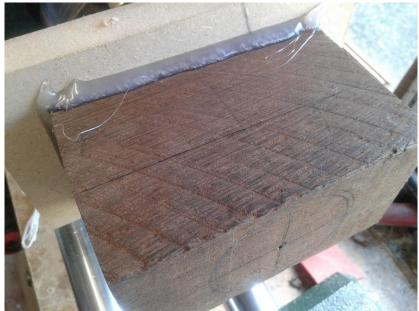
I made a very precise template of the outside of the bowl using some paper backed Walnut veneer which was less than 0.5 mm thick, but it did the job well. I also put masking tape along the line I had to stop cutting at. As it was impossible to see the pencil line whilst turning on the dark Wenge. Turning a precise half sphere was very tricky and took some time for such a small piece, a lot of stopping to check against the template. The time I took making the template definitely payed dividends.
