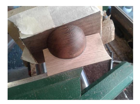
Using a wood chisel between the MDF and the back of the workpiece I parted it through the hot glue joint, it came away very easily considering the hold it had whilst turning. I then cut the piece in half on the Bandsaw.
