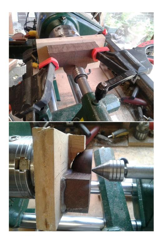
Removed the tailstock and turned out the bowl and the face. Then repeated for the second bowl.
