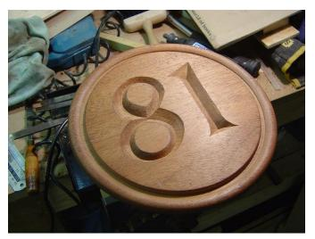
The almost finished numbers, there is still a bit of fine tuning to do but as I could still make a mess of the rope yet, I thought I would do the rope next and then do all the detail work together on the rope and numbers.
