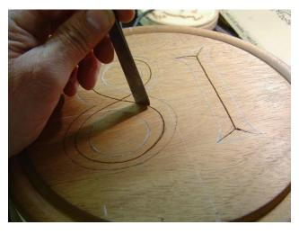
The first stage of carving the numbers is to cut a centre line, this is so when you start to carve the 'V' of the numbers the wood will not split past this centre line and possibly run past the marked line on the other edge of the numeral.
