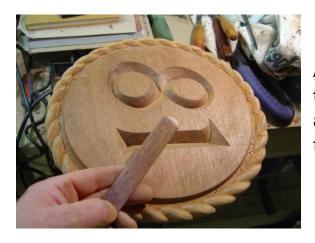
After many hours of sanding its almost there just a bit more tidy up of the rope and numbers and its ready for some finish.
