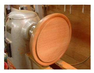
The finished stage of turning, the rim has bad the round section turned that will be carved to look like a rope wrapped around the edge of the sign.
