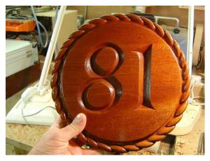
This photo shows the 3D effect of the rope better, it needs the lacquer flatted down a more coats yet. The numbers are nice and deep so should stand out nicely on the finished sign.
