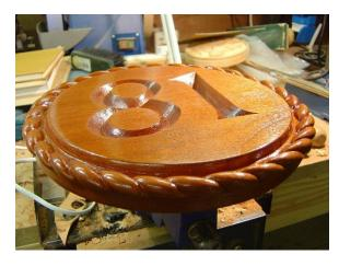
Due to the splitting issue and me not wanting to chip a section of the rope off I got to a point then moved to files and Abranet wrapped around a think lolly stick type piece of wood. This seemed to work fine and didn't have the risk of spoiling the job.
