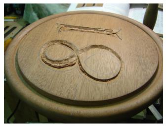
Once the centre line is cut in you then carve in at the set angle a few millimetres from each side of the centre line and the waste wood chips out along the central cut. It will take probably five or six passes to get the full width and depth of the vee.
