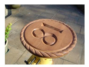
A rare sight working outside in sunlight on a hot day but better for seeing the cuts. First pass is to lightly cut the marked lines in with a vee tool.
