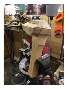
The finished band sawn blank, not looking too much like a dog yet. The dogs head and handle of the stick are one piece of wood.
