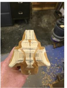
The carving is viewed from all angles constantly referring to the model for sizes. Lines are drawn on and a centre line maintained at all times for reference. The contrast in the wood colours here is the lighter sanded wood and the darker freshly cut with the gouges wood. It's given a light sand at each stage so it's easier to see the shape, when it's two tone like this it throws your eye off.
