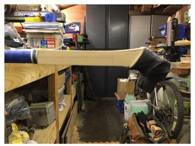
The next bit was as hard as the carving, I had finished carving on roughly square shaft that tapered to the carved area and a stick to mount it on. The only way I could shape the handle was to mount it to the stick shaft then hold it by the shaft in the vice. Then just do it all by eye, shaping with rasps, files and sand paper without spoiling the stick or carving!
