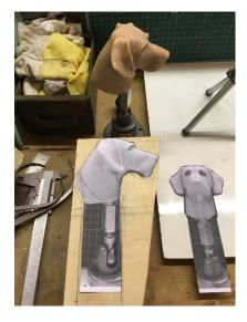
A modellers clay study is sculpted first, this is photographed from side and front and the images used to bandsaw out the lime wood blank.
