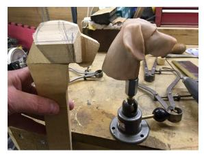
More waste Wood is removed from the band sawn blank using hand saws/ chisels. The carving is regularly checked against the model. With carving it's vital you do not take too much wood off as once it's gone it's gone and the project could be scrap.
