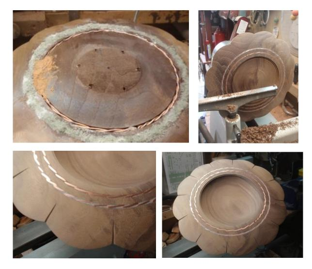
Sanding through the grits, sand off the inlay enough so the copper wire shows through. Apply a sanding sealer then the finish.
