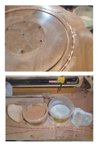
Holding the bowl in the carving jig once again I then glued the twsted copper wire in to the groove. The inlay came in rock form so I had to try and grind it in to a powder and fill over the wire with this powder. Thin CA glue was then poured over the inlay gently and allowed to soak through the soapstone and to set.
