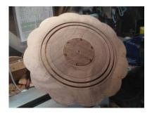
decided on the intervals for the decorative perimiter. Twelve points. Mounted on a woodcut carving jig in the banjo I marked out with a circular cotainer for each curve. Using a proxon jigsaw I then cut out the shape of the perimiter. I then remounted it on to the lathe and cut two grooves to take the copper wire and the soapstone inlay. A sanding sealer and a finish was applied to the face to stop the CA glue sinking in to the timber when puttin in the inlay.
