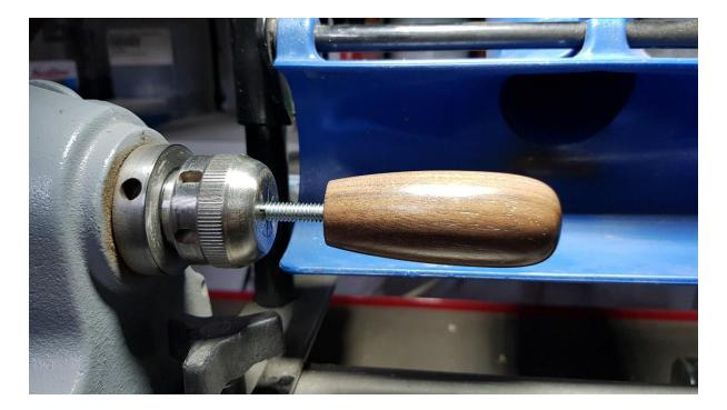
Not being one to give up on an idea easily, now that the wood has been in a centrally heated dining room for a few months, I decided to stick with acrylic lacquer. Sprayed with the lathe protected from overspray with masking tape and a scrap of hardboard.
