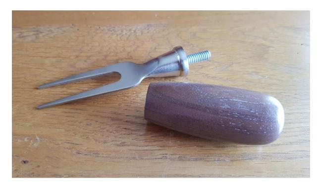
This also made them easy to mount in the collet chuck of my Axminister pen lathe using a suitable threaded rod so the old finish could be sanded away and the handles prepared for refinishing.
