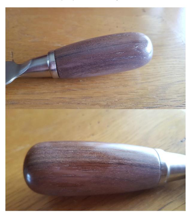
Fortunately, the handles are fitted with a screw thread so were easily removed.
