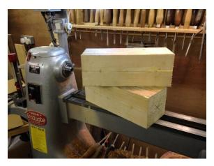
Two large blanks of pine were glued up, Jim Towers kindly planed them up to be glued for me. The project is to make two large acorns for the top of gateposts with the bottom cup section to have the criss cross pattern carved into them.
