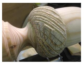
After doing all the saw cuts in one direction I found a triangle file worked best to follow in each saw cut and create a shallow vee in each groove. Tedious work! I repeated the process going the other way around doing the opposite marks, first with the saw, then first pass of the triangle file. Being right-handed one way flowed but the other didn't and using left hand didn't work either.
