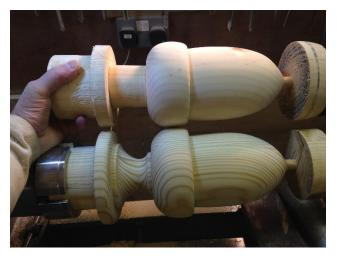
Can you spot the mistake? I had a catch and the bottom rim above the base ended up too small, I had to make a new section for under the cup and glue it on. The second acorn was then turned to match the first again.
