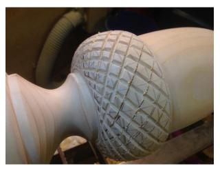
Starting to get the effect showing now, looking ok. I found that each Vee needed three passes with the file deepening them each pass, then repeating trying to keep things even by eye as they got deeper. I think it was 24 groves each direction on the layout so 48 per acorn, two acorns so 96 grooves in total, then one saw cut and three passes around with the file
