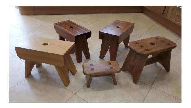
The latter three from elm. My mortice and tennon cutting was well out of practice, and I had to slacken the joints to get them to fit, which in turn created gaps. Rather than experiment with sawdust and glue as filler, I cut and glued small wedges into the gaps:
