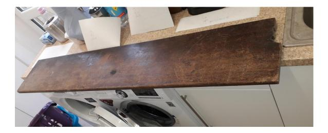
Although initially it looked like I might get two crackets out of this, on closer inspection it was riddled with screw holes resulting in unforeseen waste and I copied one of my wife's dressmaking techniques and cut paper patterns to arrange the required shapes around the defects.
